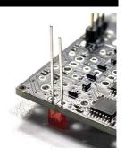
At last, put the panel on - <u>check its direction</u> - tighten the nuts and then solder all the jacks and LEDs - the closer to the panel, the more they will be evident on the panel's hollow line.
