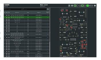
Here are listed all the TABØR components, most of them are already pre-soldered on the board. We just need to solder the through hole ones (THT).
